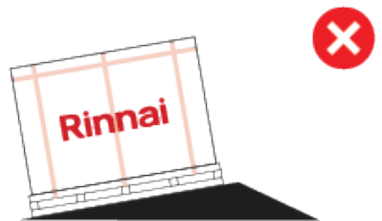
Figure 8: Do not place the Module on an uneven site
