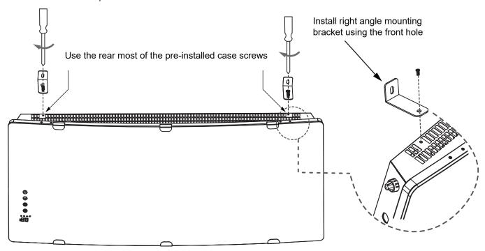
4. Hang the heater using the slots located on the back of the appliance and secure the right angle mounting brackets to the wall with appropriate fittings as shown.
