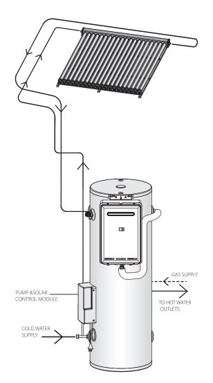
The energy the tubes collect is transferred to the consumable hot water inside the well insulated header assembly. This principle allows the collector to withstand temperatures as low as -12°C.
