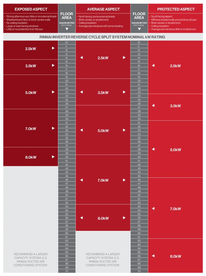
This guide has been developed to cover most normal situations. If unusual or abnormal conditions apply, a full heat load survey should be conducted.
