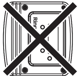
**DO NOT** install the controller on its side or back!
