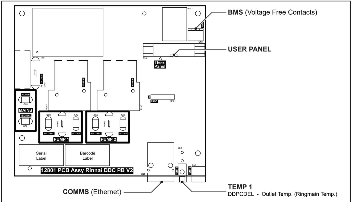
Figure 4. DDPCEDEL Internal PCB showing Thermistor Connections
