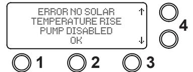
3. If one or both thermistors are outside the predetermined measurement range. This screen justifies an error with the collector short.
