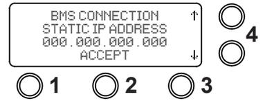
6. Using the arrow buttons select the "BMS CONNECTION STATIC IP GATEWAY 000.000.000.000" then select "ACCEPT" button 2.
