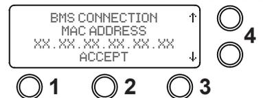
7. Using the arrow buttons select the "BMS CONNECTION RELAY NORMALLY OPEN or CLOSED" then select "ACCEPT" button 2.
