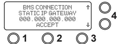
5. Using the arrow buttons select the "BMS CONNECTION STATIC IP MASK 000.000.000.000" then select "ACCEPT" button 2.
