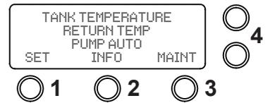
2. Using the arrow buttons select the "MEASURE RETURN TEMPERATURE YES" then select "ACCEPT" button 2.
