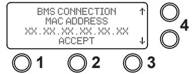
4. Using the arrow buttons select the "BMS CONNECTION RELAY NORMALLY OPEN or CLOSED" then select "ACCEPT" button 2.
