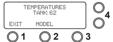
4. If the second temperature sensor has been enabled a return temperature from the HD heat source will be shown.
