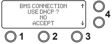
3. Using the arrow buttons select the "BMS CONNECTION STATIC IP ADDRESS 000.000.000.000" then select "ACCEPT" button 2.
