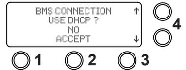
3. Using the arrow buttons select the "BMS CONNECTION STATIC IP ADDRESS 000.000.000.000" then select "ACCEPT" button 2.
