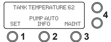
2. If one pump has been configured the pump operation status and run time hours will be displayed.
