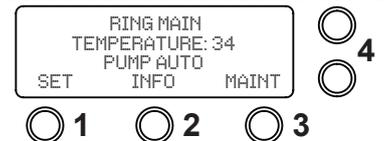
2. Using the arrow buttons select the "RING-MAIN TEMPERATURE" then select 'ACCEPT' button 2.
