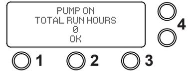
3. If two pumps have been configured the screen will scroll through pump operation status and run time hours.
