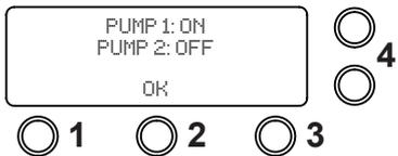
When the Ring-Main temperature is between 5°C to 10°C less the set temperature both pumps energised.
