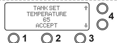
3. Using the arrow buttons select the "TANK LOW LIMIT TEMPERATURE" then select "ACCEPT" button 2.
