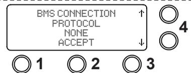
2. Using the arrow buttons select the "BMS CONNECTION RELAY NORMALLY OPEN or CLOSED" then select "ACCEPT" button 2.
