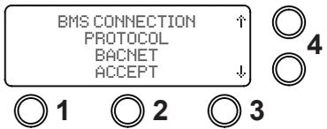
2. Using the arrow buttons select the "BMS CONNECTION USE DHCP? NO" then select "ACCEPT" button 2.
