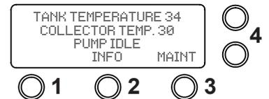
When there is a differential temperature between the solar collector (hot sensor) and the tank (cold sensor) the circulating pump is switched on. When differential falls to below the predetermined limit the circulation pump is then switched off.
