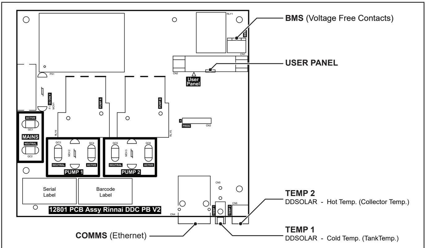
**Figure 3. DDSOLAR Internal PCB showing Thermistor Connections**
