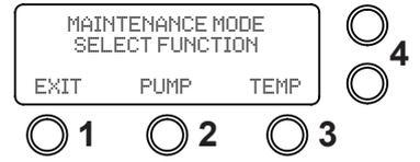
3. Use the arrow buttons to manually operate the pump on and off, select "ACCEPT" button 2 to run command.
