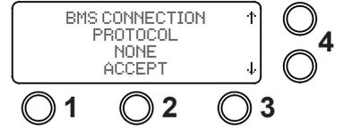
3. Using the arrow buttons select the "BMS CONNECTION RELAY NORMALLY OPEN or CLOSED" then select "ACCEPT" button 2.
