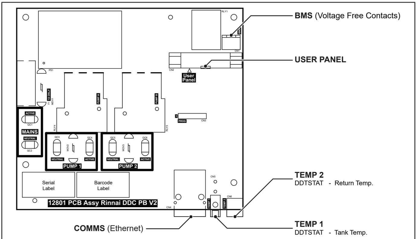
**Figure 2. DDSTAT Internal PCB showing Thermistor Connections**
