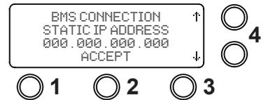
4. Using the arrow buttons select the "BMS CONNECTION STATIC IP GATEWAY 000.000.000.000" then select "ACCEPT" button 2.
