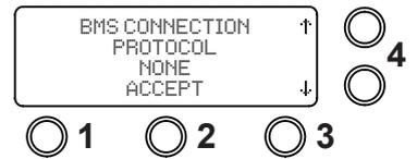
2. Using the arrow buttons select the "BMS CONNECTION PROTOCOL NONE" then select "ACCEPT" button 2.
