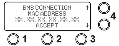
6. Using the arrow buttons select the "BMS CONNECTION RELAY NORMALLY OPEN or NORMALLY CLOSED" then select "ACCEPT" button 2.
