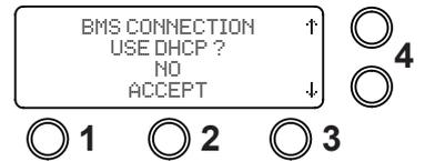
5. Using the arrow buttons select the "BMS CONNECTION STATIC IP ADDRESS 000.000.000.000" then select "ACCEPT" button 2.
