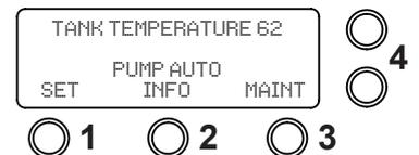
2. Using the arrow buttons select the "TANK SET TEMPERATURE" then select "ACCEPT" button 2.
