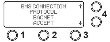
4. Using the arrow buttons select the "BMS CONNECTION USE DHCP? YES" then select "ACCEPT" button 2.
