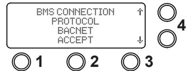
2. Using the arrow buttons select the "BMS CONNECTION USE DHCP? NO" then select "ACCEPT" button 2.
