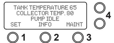
2. The screen will alternate between pump operation status and run time hours.
