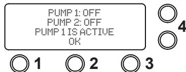
When Ring-Main temperature within 5°C less of set point, one pump is operational.
