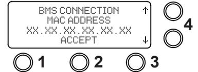
4. Using the arrow buttons select the "BMS CONNECTION RELAY NORMALLY OPEN or CLOSED" then select "ACCEPT" button 2.
