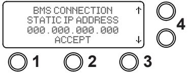
4. Using the arrow buttons select the "BMS CONNECTION STATIC IP GATEWAY 000.000.000.000" then select "ACCEPT" button 2.
