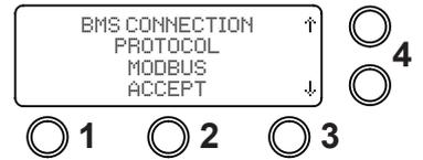
4. Using the arrow buttons select the "BMS CONNECTION USE DHCP? NO" then select "ACCEPT" button 2.
