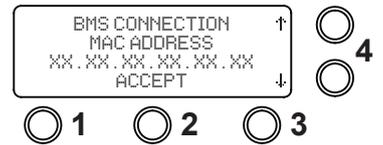
6. Using the arrow buttons select the "BMS CONNECTION RELAY NORMALLY OPEN or CLOSED" then select "ACCEPT" button 2.
