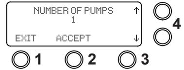
3. Using the arrow buttons select the "ALTERNATE PUMP OPERATION YES" then select "ACCEPT" button 2.
