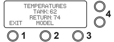
4. The Controller configuration will then be displayed select "EXIT" button 2 to return to home screen.
