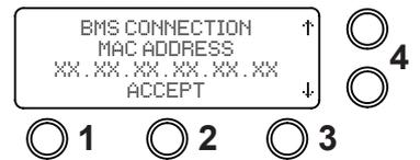
9. Using the arrow buttons select the "BMS CONNECTION RELAY NORMALLY OPEN or NORMALLY CLOSED" then select "ACCEPT" button 2.
