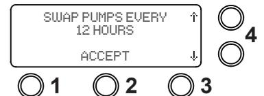
5. From "CONTINUE TO ADVANCED SETUP" screen select "YES" button 3 to continue to set up BMS connectivity or "NO" button 1 to finalise and exit.
