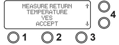
3. Using the arrow buttons select the "RETURN TEMP LOW LIMIT" then select "ACCEPT" button 2.
