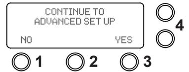
3. Using the arrow buttons select the "BMS CONNECTION PROTOCOL MODBUS" then select "ACCEPT" button 2.
