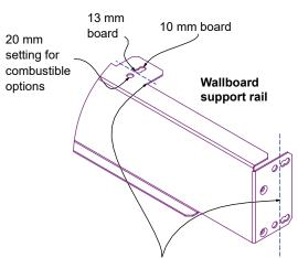
**Note**: Wallboard support rails, the tabs for 10 mm and 13 mm boards need to be trimmed off as indicated. If not using the optional Outer Finishing Trim around the edge of the wallboard, then the latches can be snapped off, otherwise the wallboard support rails and wallboard will need to have clearance applied to fit.
