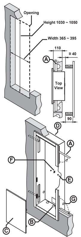
7. To help reduce the risk of theft or damage, attach the supplied padlock to the padlock tab (F) as required.
