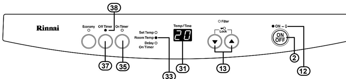
To operate, press the Off Timer button (37). The Off Timer indicator (38) will illuminate and the Combustion indicator (12) will be illuminated red to confirm that the heater will continue operation until the Delay 'off' time period has passed after which it will stop. The Delay Off time is 60 minutes. When this time has passed, the heater will automatically stop operation and the Off Timer indicator (38) will flash.
