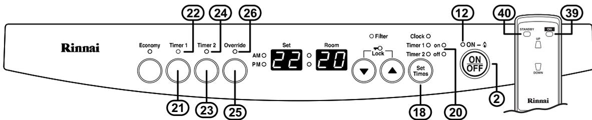
The heater must be between the finishing and starting times of a timer program for the Override to function to work. Either of the Timer indicators (22) or (24) will be illuminated and the Combustion indicator (12) is illuminated green when this is the case. If the Override button (25) is pressed the Override indicator (26) will flash to show that the heater is now operating in override mode. The heater will now start and full manual control will now be available.
