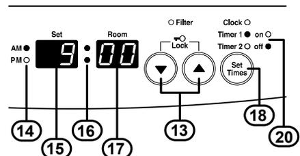
The factory default Timer 1 'Off' time is AM 09:00. Press the Up or Down buttons (13) to adjust the Timer 1 'Off' time.
