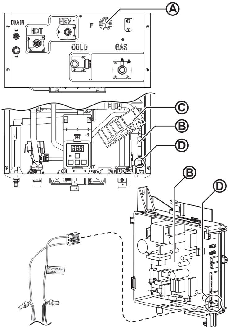
**UNIVERSAL WATER CONTROLLER (MC-601Q) INSTALLATION**
