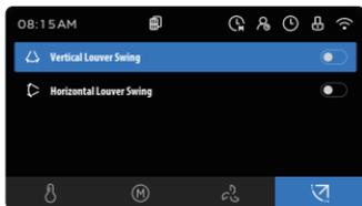
2. Press “ $\hat{+}$ ” or “ $\hat{-}$ ” to select the fan direction function, press “ $\checkmark$ ” to enable or disable the function; whether there is a fan direction function is determined by indoor unit.
