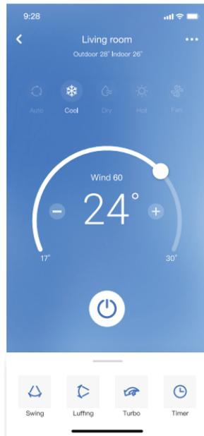
3. Touch to turn on. The user can control the AC on/off status, operation mode, fan speed, temperature, etc.
