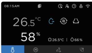
3. When Horizontal Louver Swing\* is selected, press “ $\checkmark$ ” to enable/disable the Horizontal Swing\* function.
