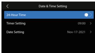
2. The time setting interface of the wired controller is as follows:
