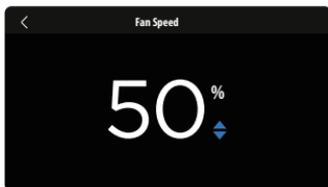
4. In stepless speed regulation Setting state, press “ $\hat{+}$ ” or “ $\hat{-}$ ” to adjust the Fan speed, the setting range is 1%~100%.
