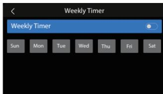
2. Use “ $\wedge$ ”, “ $\vee$ ”, “ $<$ ” or “ $>$ ” to select the timer date, and use “ADD” to add the set time, include Timer On, Timer Off, Temp, Mode, Fan Speed.
