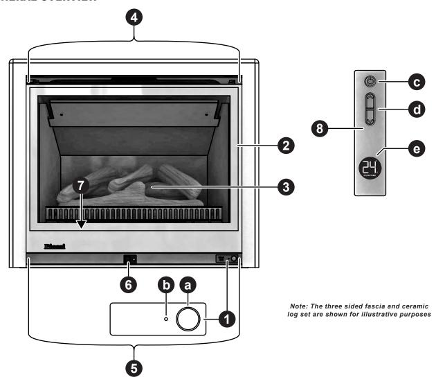
Push button control panel Controls appliance operation between Standby and ON modes.
