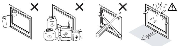
**DO NOT** spray aerosols in the vicinity of this appliance whilst the heater is operating. Most aerosols contain flammable gas, which can be a fire hazard if used near the heater when it is in use.
