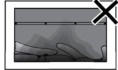
SOOT BUILD UP
