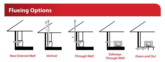
**Please note:** \*Suitable for direct, vertical or horizontal flueing. 500mm required for down and out applications. See installation instructions for full details.
