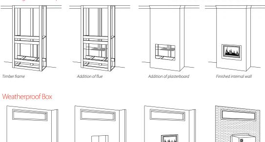
For an alternative installation to a false fireplace, the Rinnai 950X can be installed into a weatherproof box. A cavity is cut into the existing blank wall and the fireplace is installed onto a bracket that allows the back of the fire to sit outside housed in a tightly sealed box. This option allows the fire to be built into an existing wall without taking up any extra space in the room. The weatherproof box is sold separately.
