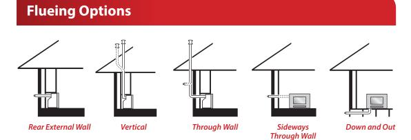
Please note: Suitable for direct, vertical or horizontal flueing. 500mm required for down and out applications. See installation instructions for full details.
