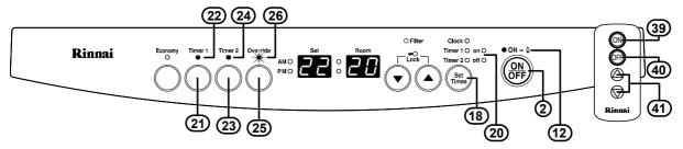
The heater must be between the finishing and starting times of a timer program for the Override to function to work. Either of the Timer indicators (22) or (24) will be illuminated and the Combustion indicator (12) is illuminated green when this is the case. If the Override button (25) is pressed the Override indicator (26) will flash to show that the heater is now operating in override mode. The heater will now start and full manual control will now be available.
