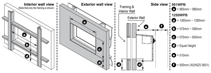
Prepare framing and cavity in accordance with all Local Regulations and Municipal Building Codes including local OH&S requirements. The joists used to support the appliance off the ground **MUST BE** capable of supporting a minimum of 105kg.
