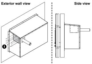
Secure the side (air hose) access panel I to the box (PH screws x9).
