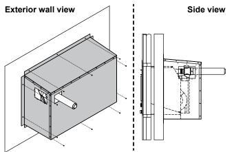
Secure the box assembly to the exterior wall (with appropriate fixings), ensuring that it is both level and symmetrically aligned with the cavity / penetration, the heater support shelf and the appliance.
