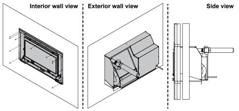
Mount and secure the appliance and connect the flue system in accordance with the OPERATION & INSTALLATION MANUAL, Power Flued Flamefire Gas Space Heater RHFE-951ETR / 1250ETR (supplied with the heater) and the INSTALLATION MANUAL, Power Flued Flamefire Space Heater Co-Axial Flue System (supplied with the flue).
