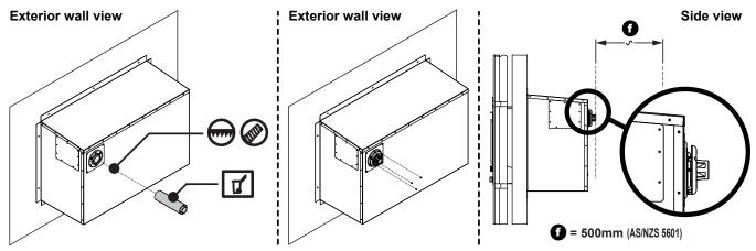
Prepare flue pipe and install flue terminal components in accordance with INSTALLATION MANUAL, Power Flued Flamefire Space Heater Co-Axial Flue System (supplied with the flue).
