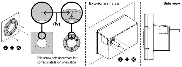
With the screw hole (iv) uppermost, secure the flue terminal wall plate K (supplied with the flue terminal) to the rear (flue) access panel J (SD screws x3), then with the same orientation fit this assembly over the flue pipe and secure it to the box (SD screws x4).
