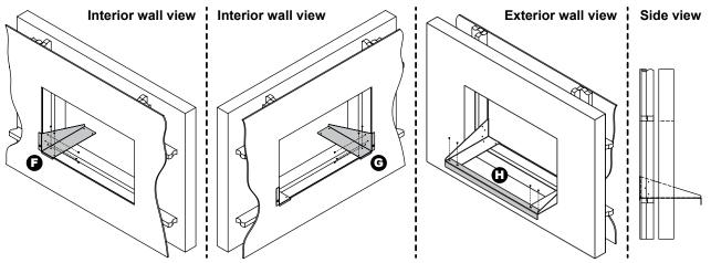
Fit side shelf bracket **F** to the bottom left corner of the framing so that the return folds are flush with the interior wall, secure in place (W screws x5). Repeat for side shelf bracket **G** in the opposite corner. Fit the L shaped cross brace **H** over the rear of side self brackets, with the tab facing downwards and secure to make rigid (PH screws x4).
