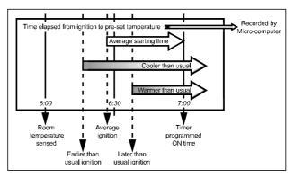
The temperature differential at the time of sensing the room temperature combined with the data from previous operation governs exactly how long before the programmed On time the micro-computer will operate the heater and ignite the burner.
