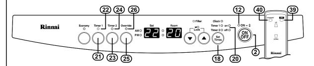
The heater must be between the finishing and starting times of a timer program for the Override to function to work. Either of the Timer indicators (22) or (24) will be illuminated and the Combustion indicator (12) is illuminated green when this is the case. If the Override button (25) is pressed the Override indicator (26) will flash to show that the heater is now operating in override mode. The heater will now start and full manual control will now be available.
