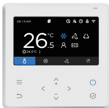
Power-on status main page display
